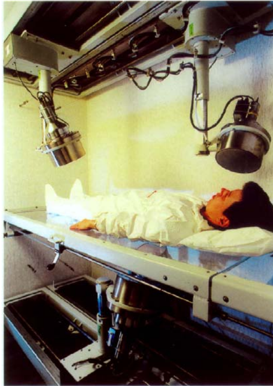
Body counter of the Karlsruhe Institute of Technology (KIT) to determine the gamma-radiating radionuclides in the human body
